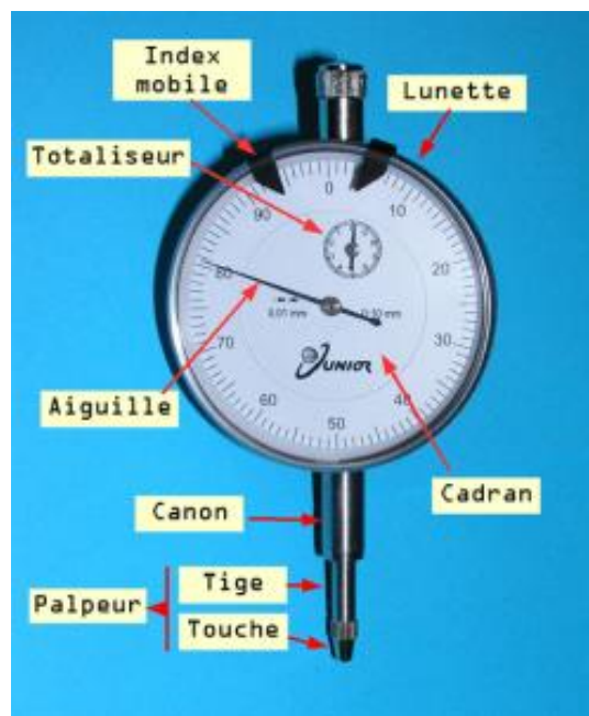
Figure 2.2.8. Schematic view of a comparator
