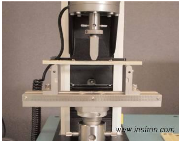
Figure 2.3.2. Example of three-point bending test
